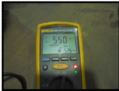
Fig 47. Insulation W1-G Test
