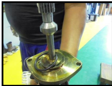
Fig 20. Cleaning Gear Torque Switch
