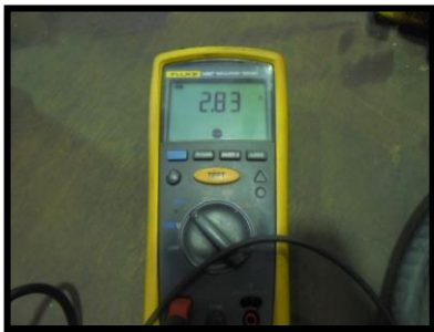
Fig 44. Coil Resistance 3 Test
