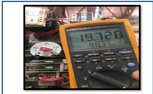
Fig 6. Feedback Signal 100% (Before)
