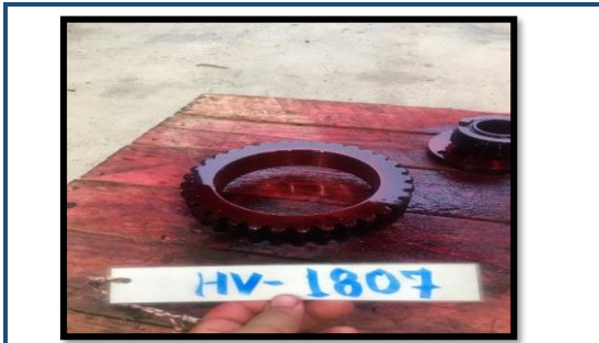
Fig 25. Inspection by Penetrant Testing ( PT Test ) Worm Gear
