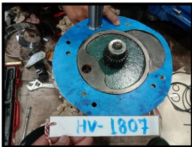
Fig 35. Change New Gasket
