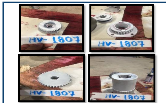
Fig 28. Inspection by Penetrant Testing ( PT Test ) Gear Shaft Motor
