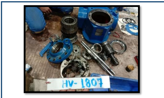
Fig 7. Remove Actuator at Shop
