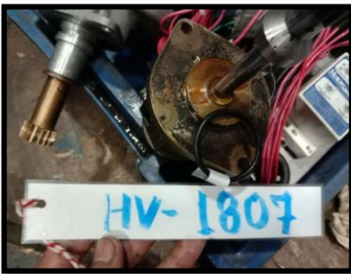
Fig 31. Change New O-ring
