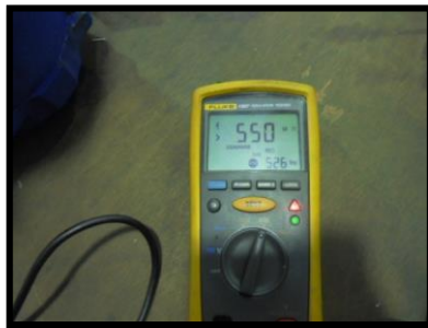
Fig 45. Insulation U1-G Test
