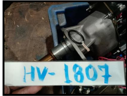
Fig 30. Change New O-ring
