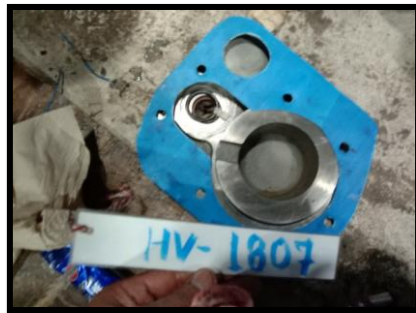
Fig 32. Change New O-ring
