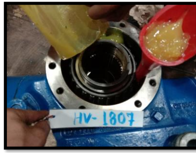
Fig 38. Change New Grease
