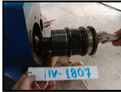
Fig 10. Inspect Spring Torque
